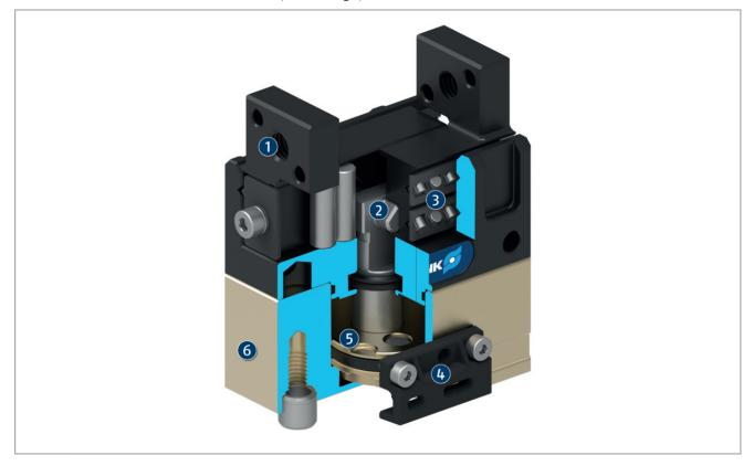
The oval piston is moved up or down by compressed air. The angled active surfaces of the wedgehook produce a synchronized, parallel jaw motion.
