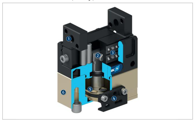
The oval piston is moved up or down by compressed air. The angled active surfaces of the wedge-hook produce a synchronized, parallel jaw motion.
