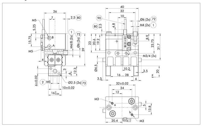
The drawing shows the basic version of the gripper with open jaws, without dimensional consideration of the options described below.
