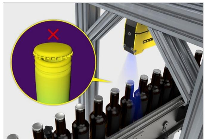
Ensure the bottle is properly sealed by checking the height and tilt angle of the bottle cap.
