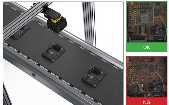
**Verify proper insertion of components**
