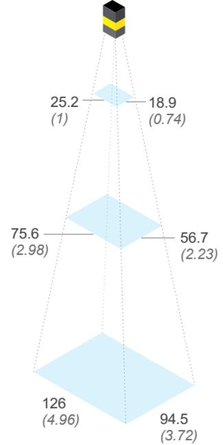
\*Applications with working distances beyond 500 mm may result in an in-focus image but light uniformity/intensity will be significantly lower. External lighting is recommended for these scenarios.
