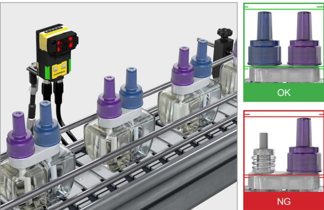
**Inspect for mechanical defects**
